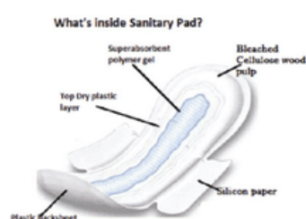
Figure: Different layers of a typical sanitary pad (Source: www.scienceandsamosa.com )
